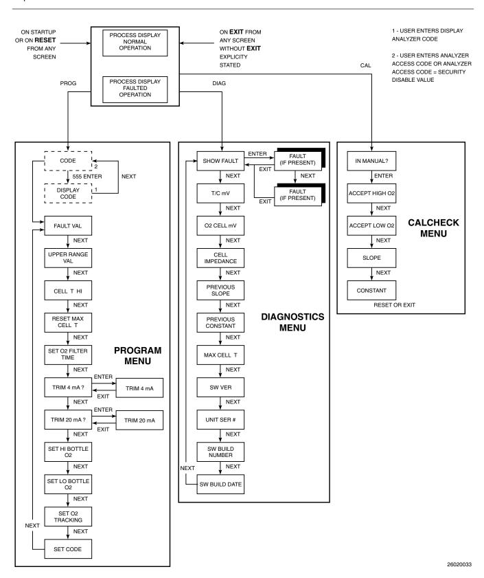
Figure 3-5. Model 3081 Transmitter Menu Tree
